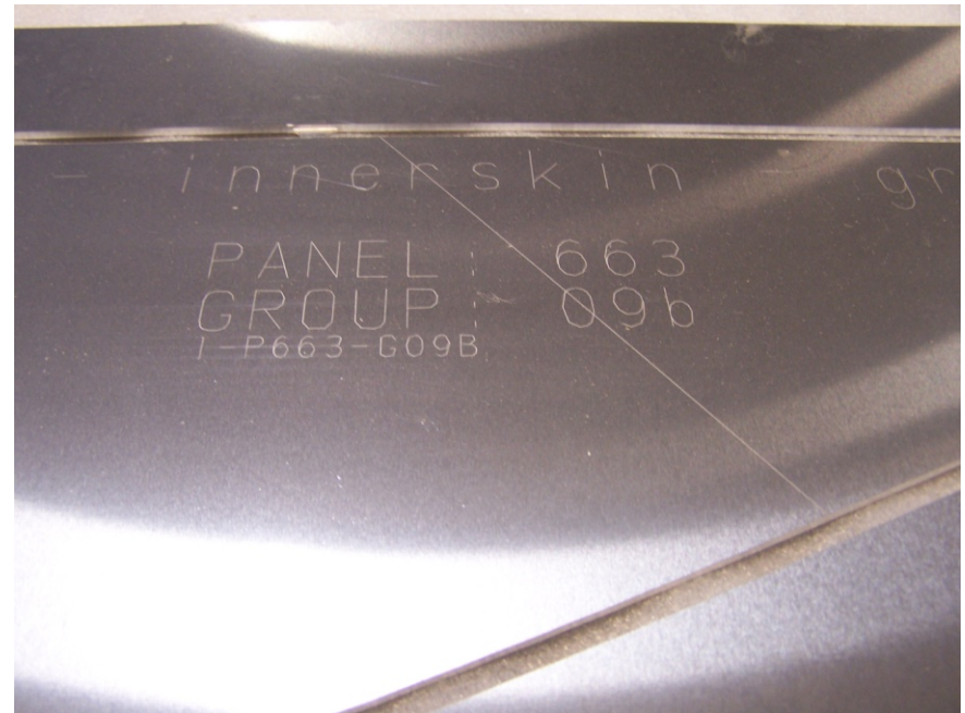
Figure 6. Top-left: The 2D CNC machine used to cut all of the panels. Top-right: The panels cuts were perforated so they could be delivered attached to the sheet they were cut out of. They were then snipped out for assembly as needed. Bottom-right: a label created by the CNC laser etching head indicating panel type, panel number, and group number. Bottom-left: A working surface with a 1-foot grid to assist alignment during assembly.
