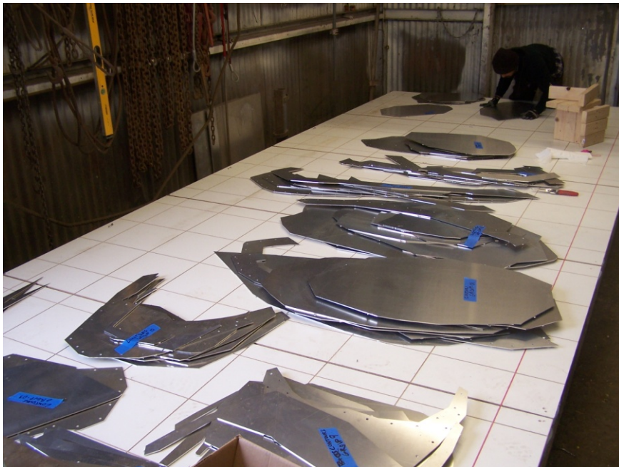
Figure 6. Top-left: The 2D CNC machine used to cut all of the panels. Top-right: The panels cuts were perforated so they could be delivered attached to the sheet they were cut out of. They were then snipped out for assembly as needed. Bottom-right: a label created by the CNC laser etching head indicating panel type, panel number, and group number. Bottom-left: A working surface with a 1-foot grid to assist alignment during assembly.
